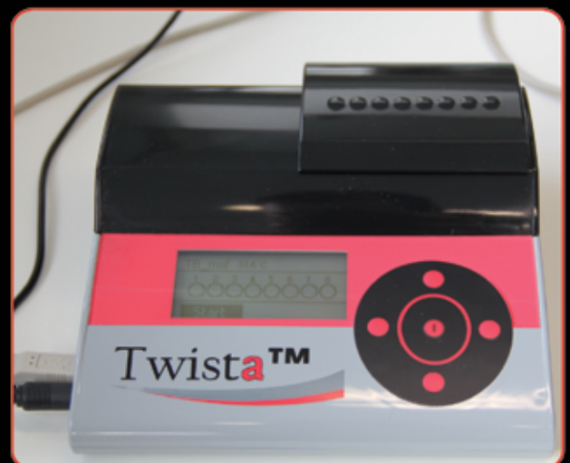
d. Real time portable heated fluorometer; The Twista™ or any real-time PCR machine
