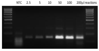
Fig.1 DNA amplification using TwistAmp<sup>®</sup> Basic reactions (250 copies positive control) at incubation temperature of 40 °C, 2% agarose gel, \* 100% of all samples loaded except 100/200ml reactions where 50µl was cleaned up and ran on gels. No template control (NTC) was a 50µl reaction.
