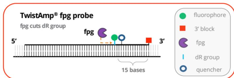
**Figure 8.** Schematic of the structure of an annealed TwistAmp® fpg probe. The abasic dR residue is cleaved by fpg only when the probe is bound to its target. This cutting step releases the fluorophore from the probe and the quencher proximity and generates fluorescence signal.
